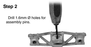
Drill & break through from top and then bottom. Then gently run drill right through to align both holes. Step 3
